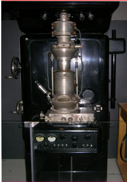
Figure 4 Electron microscope constructed by Ernst Ruska (1933)
