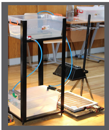
Fig.3. The module "PV and energy storage via water"
