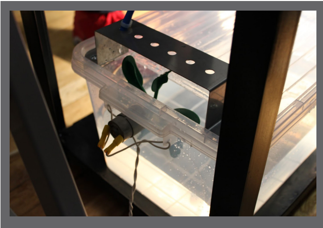
Fig.5. Microturbine and electric generator
