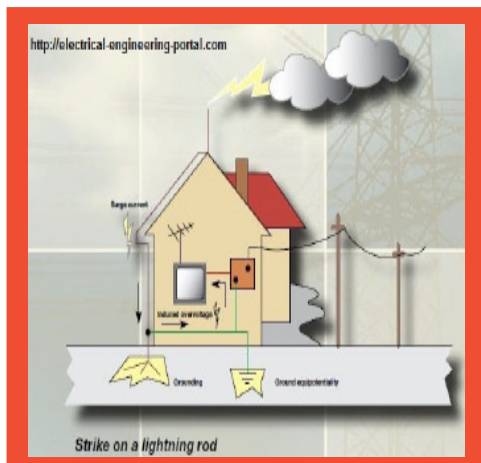
Fig. 4. Functioning of a Lightning rod
