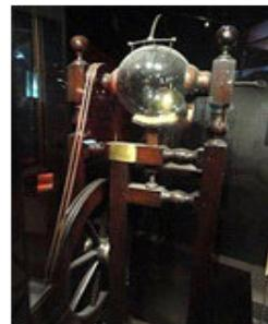
Fig. 8 Franklin's electrostatic machine
