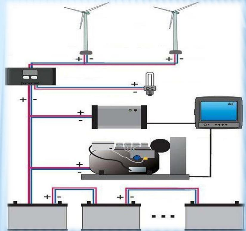
In this image is presented a power production system that includes a generator powered by a thermal engine.
